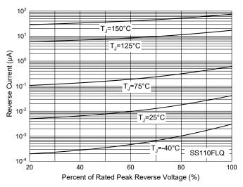
Fig. 6 - Typical Reverse Leakage Characteristics
