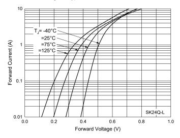
Fig. 5 - Typical Forward Characteristics
