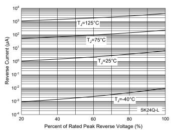
Fig. 6 - Typical Reverse Leakage Characteristics
