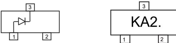
**350mW 100 Volt Silicon Epitaxial Diode**
