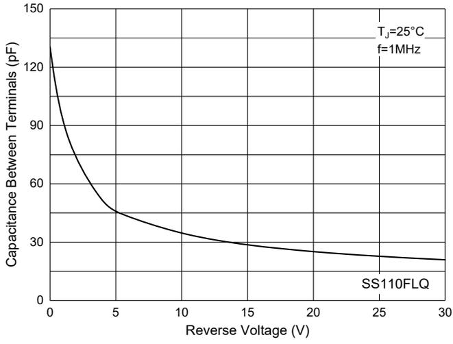
Fig. 8 - Capacitance Characteristics
