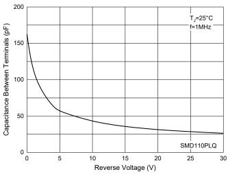
Fig. 7 - Capacitance Characteristics
