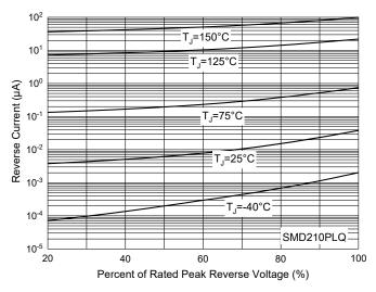
Fig. 6 - Typical Reverse Leakage Characteristics
