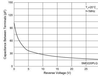
Fig. 8 - Capacitance Characteristics
