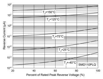
Fig. 6 - Typical Reverse Leakage Characteristics
