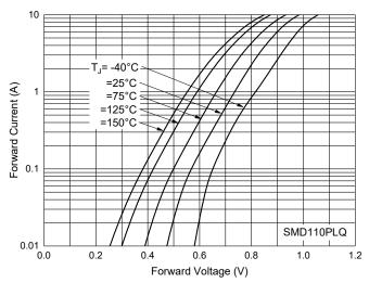
Fig. 5 - Typical Forward Characteristics
