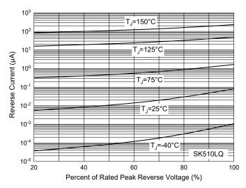
Fig. 6 - Typical Reverse Leakage Characteristics
