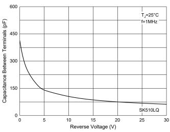
Fig. 7 - Capacitance Characteristics
