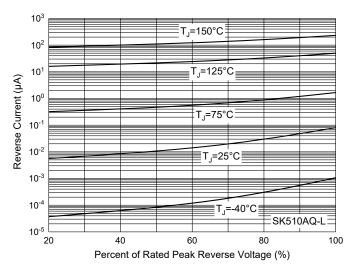
Fig. 6 - Typical Reverse Leakage Characteristics
