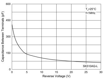
Fig. 7 - Capacitance Characteristics
