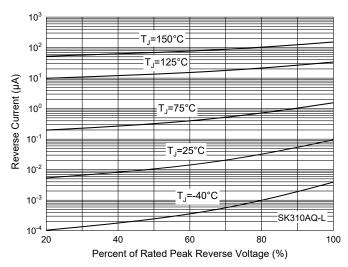
Fig. 6 - Typical Reverse Leakage Characteristics
