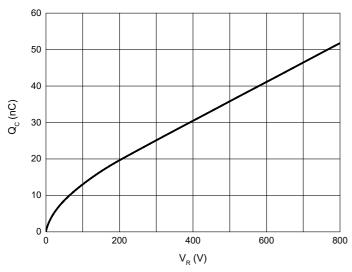
Fig. 6 - Capacitance Stored Energy
