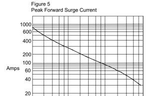
Peak Forward Surge Current - Amperesversus Pulse Duration - Milliseconds (mS)
