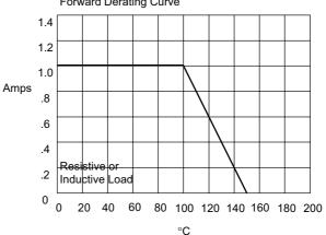
Average Forward Rectified Current - Amperes/ersus Ambient Temperature - $^{\circ}$ C
