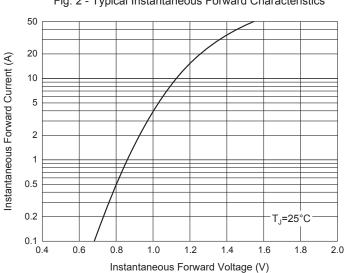
Fig. 2 - Typical Instantaneous Forward Characteristics
