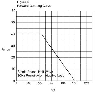
Average Forward Rectified Current - Amperes/ersus Ambient Temperature  $\ \ \circ^{\rm C}$
