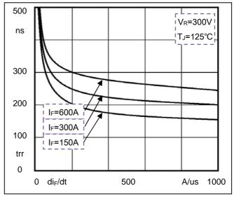
Fig2. Reverse Recovery Time vs di<sub>F</sub>/dt
