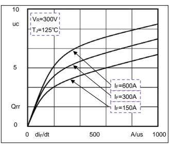
Fig4. Reverse Recovery Charge vs di<sub>F</sub>/dt
