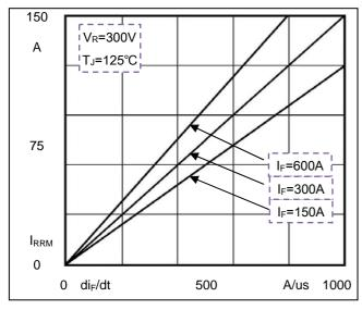
Fig3. Reverse Recovery Current vs di<sub>F</sub>/dt
