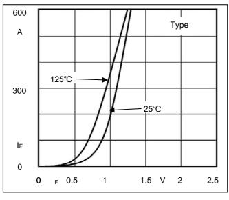
Fig1. Forward Voltage Drop vs Forward Current
