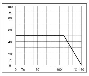
Fig5.Forward Current Derating Curve
