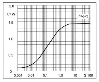
Fig3. Transient thermal impedance
