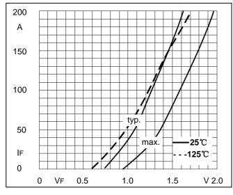
**Fig1. Forward Characteristics**
