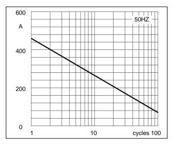
Fig4. Max Non-Repetitive Forward Surge Current
