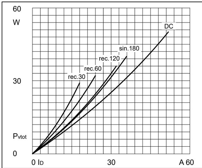
**Fig1. Power dissipation**
