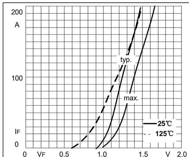
**Fig5. Forward Characteristics**
