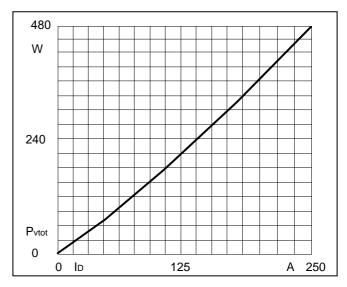
Fig2. Power dissipation
