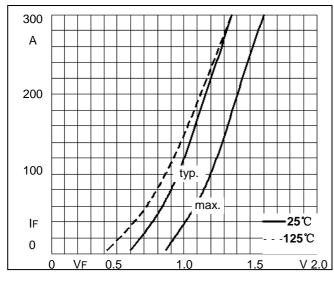
**Fig1. Forward Characteristics**
