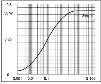
Fig3. Transient thermal impedance
