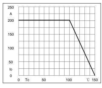
Fig5.Forward Current Derating Curve
