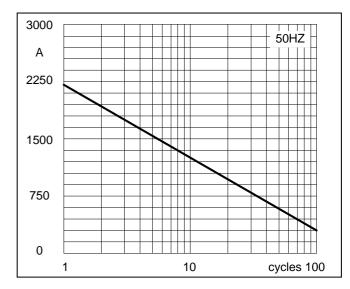
Fig4. Max Non-Repetitive Forward Surge Current
