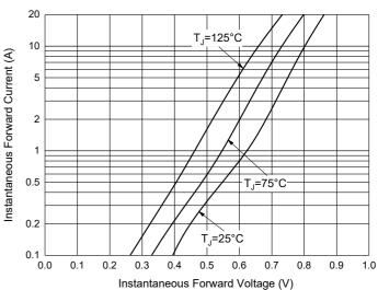
Fig. 2 - Typical Instantaneous Forward Characteristics
