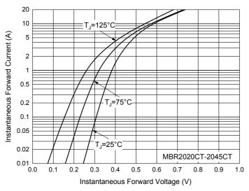
Fig. 5 - Typical Instantaneous Forward Characteristics
