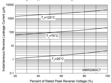
Fig. 8 - Typical Reverse Leakage Characteristics
