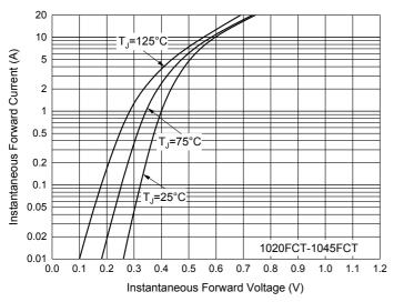
Fig. 5 - Typical Instantaneous Forward Characteristics
