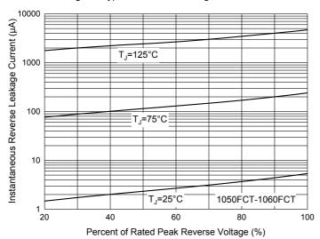
Fig. 8 - Typical Reverse Leakage Characteristics
