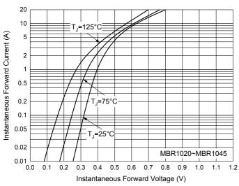
Fig. 5 - Typical Instantaneous Forward Characteristics
