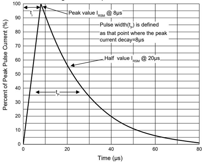
**Fig. 2 - Non-Repetitive Peak Pulse Power**
