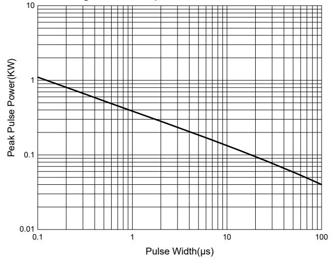
Fig. 2 - Non-Repetitive Peak Pulse Power
