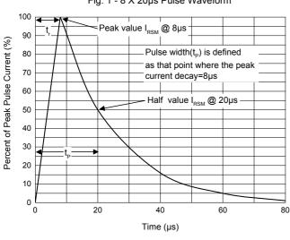
Fig. 1 - 8 X 20µs Pulse Waveform
