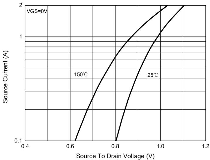
Fig. 10 - Drain Current
