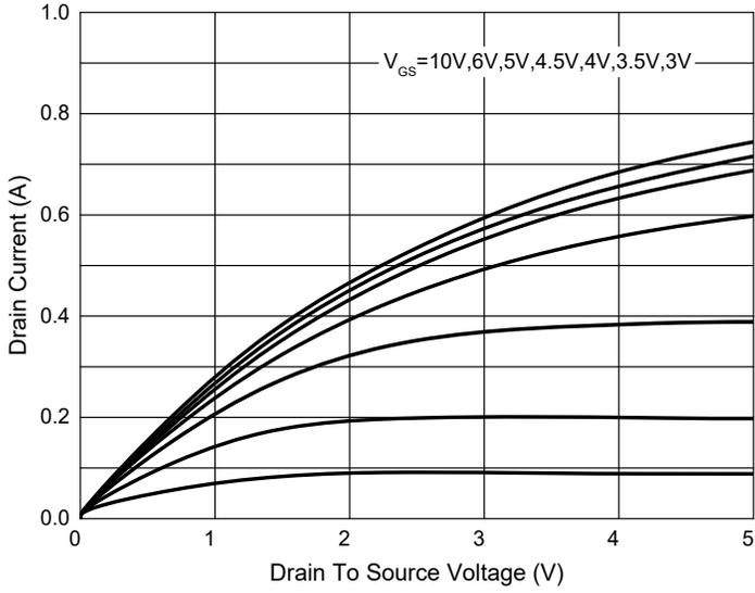
Fig. 2 - Transfer Characteristics
