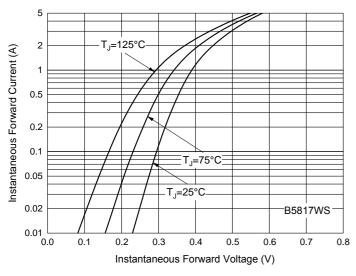
Fig. 5 - Typical Instantaneous Forward Characteristics
