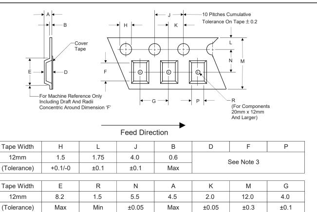
Note 3: D,E,F are determined by constant size. The clearance between the part and the tape cavity must be within 0.05mm min. to 0.65mm max. for 12mm tape.
