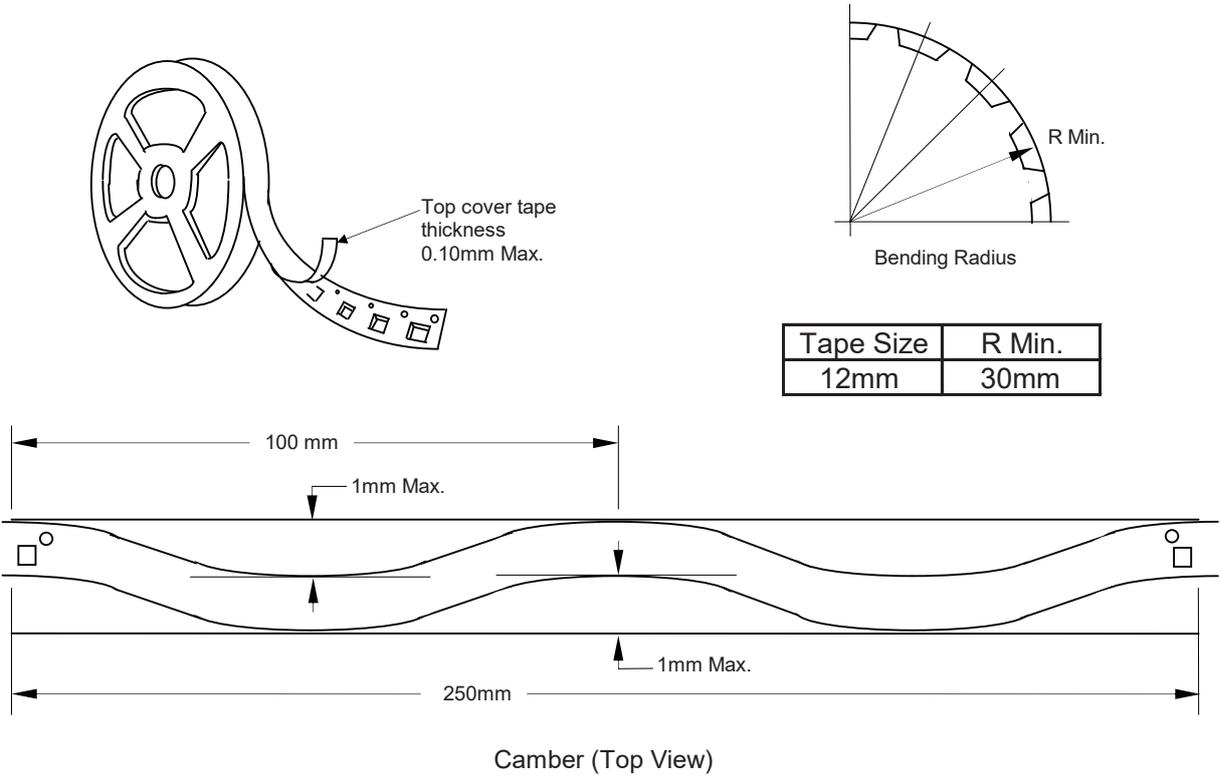
Allowable camber to be 1mm/100mm non-accumulative over 250mm
