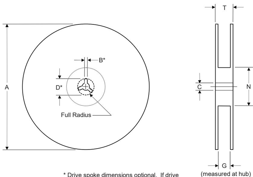
\* Drive spoke dimensions optional. If drive spoke is used then asterisked dimensions apply.
